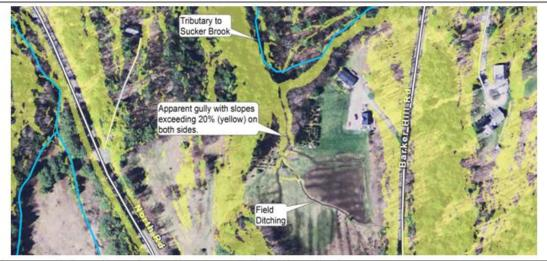
Photo 1: Aerial photo of site with steep slopes (>20%) highlighted in yellow from LiDAR.
